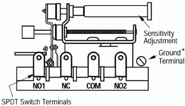
\*The internal ground connection is only available on the VS2 by threading the nut supplied in the hardware kit onto the base mounting bolt.
