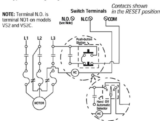
**VS2, VS2C, VS2EX, VS2EXR, VS2EXRB and VS94**
