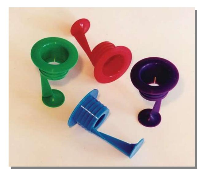
Star Cooling Towers Precision-Flo water distribution nozzle is a non-clogging nozzle designed specifically for all crossflow cooling tower applications. It provides excellent flow characteristics utilizing a one piece design with single support distribution plate. This produces a uniform distribution pattern helping to enhance the cooling tower's thermal performance.
