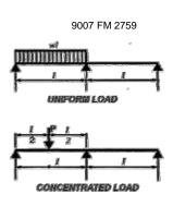
$beam\ spanning\ two\ equal\ lengths\ with\ the\ uniform\ or\ concentrated\ load\ on\ one\ span\ only,\ multiply\ the\ above\ deflections\ by\ 0.71.$
